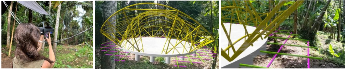
Figure 3. AR display of design intent for in-situ decision-making of orientation and exact localisation.
